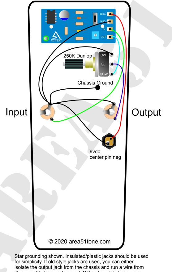
it's ground to the input ground, OR just omit that wire and connect both jack sleeves to the chassis with internal tooth washers. Either way will work, but the isolated jack/star ground method could be less prone to pick up noise.
